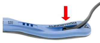
2. Simultaneously push the wide end of spring into receiver slot (arrow 1) and rotate thin knob end up (arrow 2).
