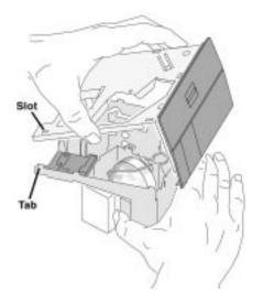
Insert the remainder of the **tabs** into slots until all 7 tabs on the top and 2 on the bottom are secured. Insert the screw and tighten. Then insert and seat the lamp.
