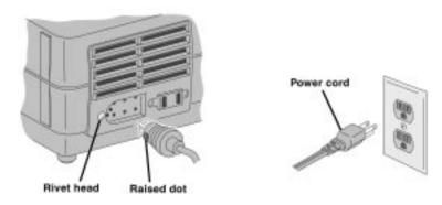
Plug the **power cord** into a grounded outlet with 110- to 125-volt 60 Hz current only.
