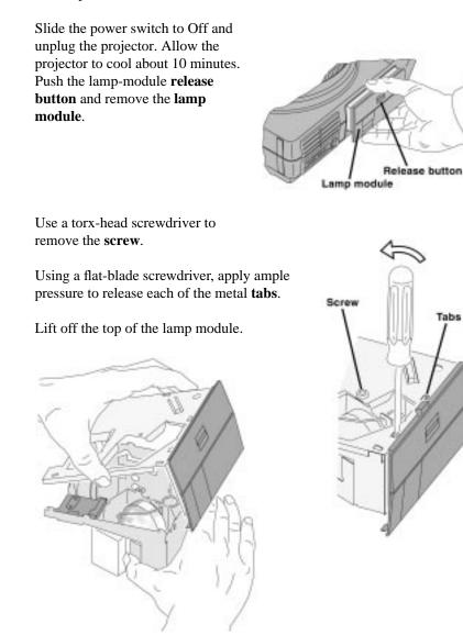
To clean the condenser, heat-absorbing glass, or mirror, you must disassemble the lamp module.
