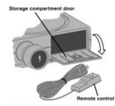
Plug the 5-pin cable remote connector into the remote-control receptacle, aligning the **raised dot** with the metallic **rivet head**.
