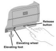
If the image is not level, make an adjustment by turning the **leveling foot** at the rear of the projector.
