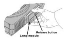
Lift up the **lamp release clip**. Carefully remove the worn **lamp** from the socket and place it on a heat-resistant surface.
