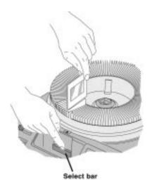
Adding a Slide When the lock ring is off, you can add a slide to any empty slot. (See "Adding Your Slides" on page 6.)
