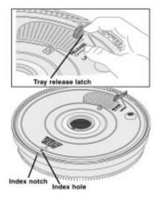
With the lock ring firmly in place, turn the 140-slide tray upside down. Retract the **tray release latch** in the direction of the arrow and align the **index hole** with the **index notch**. (For an 80-slide tray, rotate the metal plate until it locks into position.) Put the tray aside.
