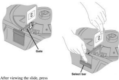
forward, reverse, or the **select bar** to eject the slide.
