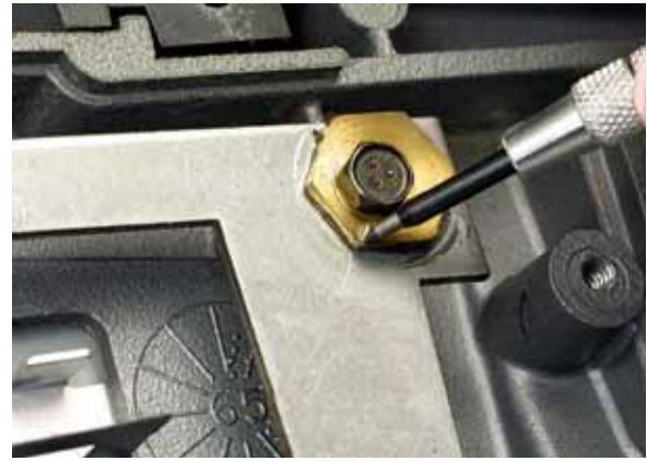
FIG. D15 Scribing the eccentric bearing for the forward/reverse arm.
