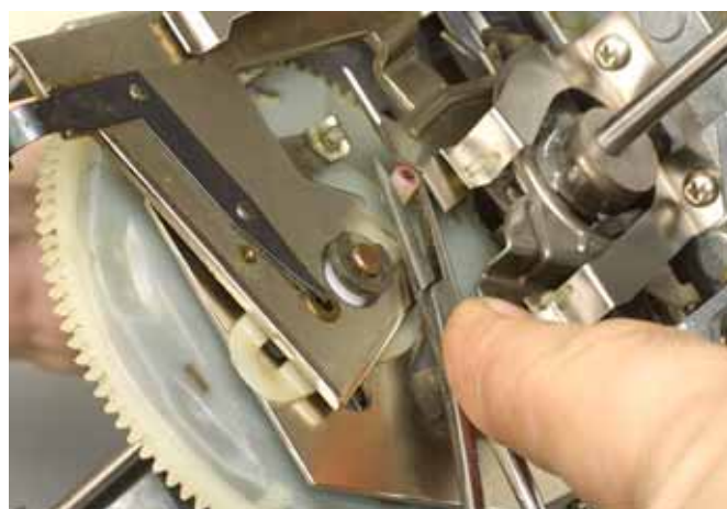
FIG. D83 Replacing the followers at the front of the in-and-out cam.
