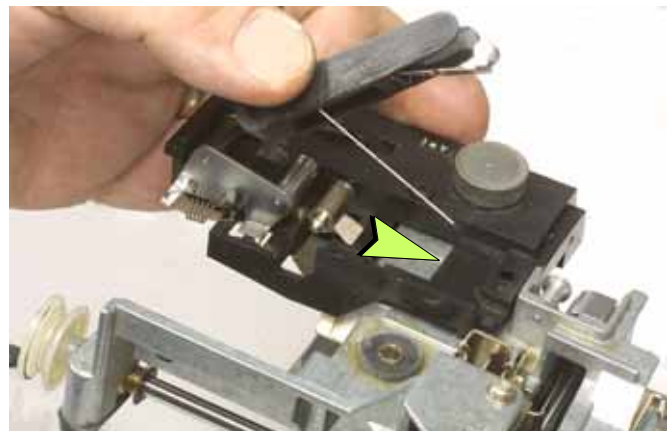
FIG. D91 The damping arm in position for inserting the flat spring through the cover slot.
