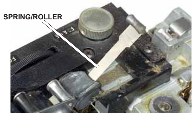
FIG. D89 A broken damping arm viewed from the back of the mechanism.
