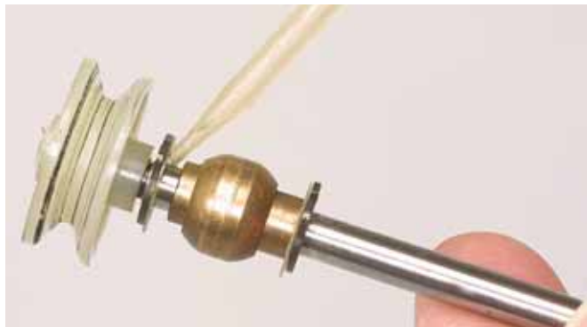
FIG. D59 Lubricating the shutter-drive shaft.
