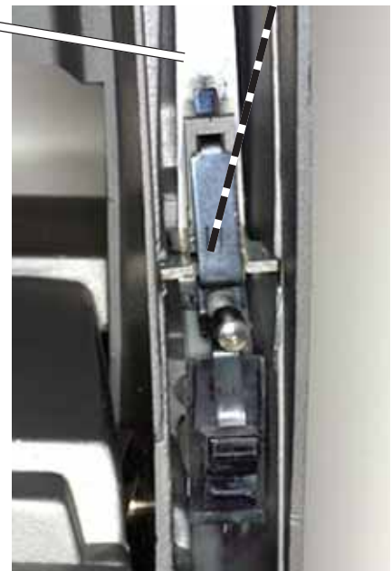
FIG. D113 Mechanism that moves the rewind driver to engage the supply reel.
