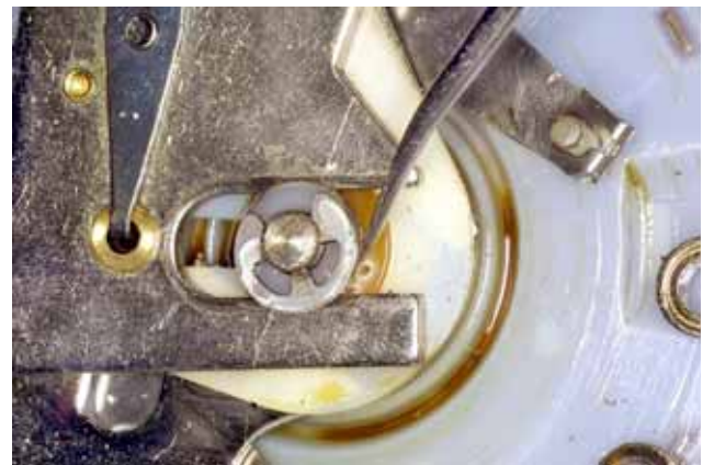
FIG. D37 Probing the cam-shaft bushing to test its condition. This one needs to be replaced.
