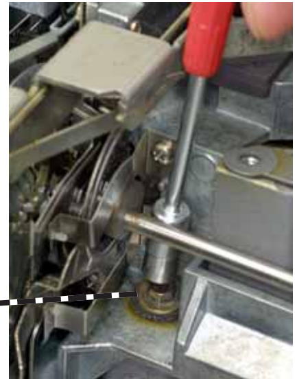
FIG. D30 Using a thin-walled 1/4" nut driver to remove the third mechanism screw.
