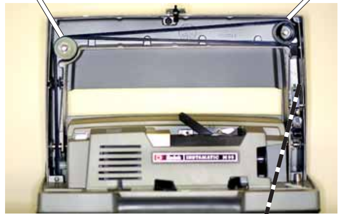
FIG. D111 Front of projector with cover plate removed.
