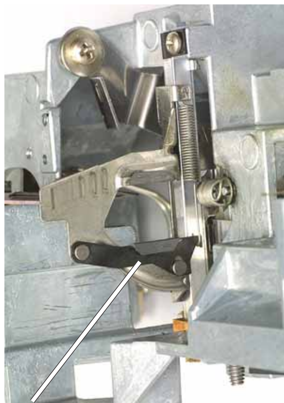
FIG. D61 Installation position for the M80 shutter-drive shaft—start with the large lobe on the dashed line and then turn the shutter-drive shaft clockwise to the position shown.
