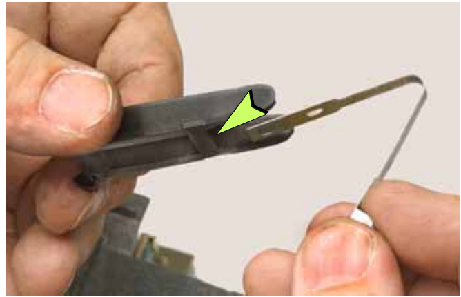
FIG. D90 Installing the spring/roller unit in the new damping arm.
