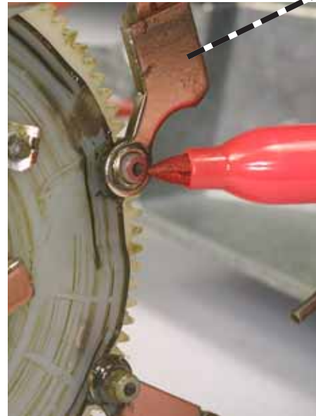
FIG. D43 Marking the super-8 follower with a felt-tip pen.
