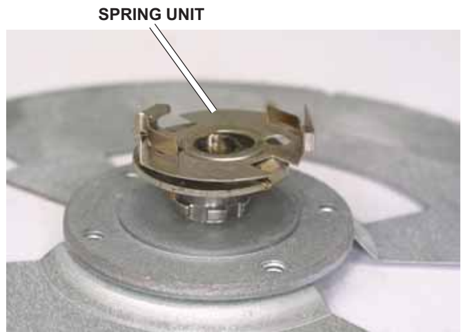
FIG. D57 Spring unit at the front of the shutter. This one is already loose.
