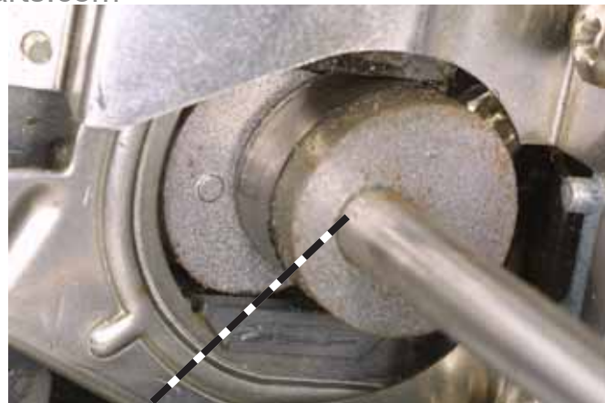
FIG. D61 Installation position for the M80 shutter-drive shaft—start with the large lobe on the dashed line and then turn the shutter-drive shaft clockwise to the position shown.
