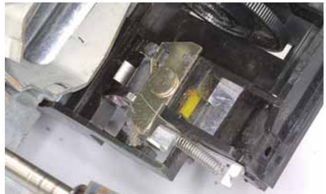
FIG. D96 Variation in the latching mechanism for the damping arm. Here the spring does not disconnect when you remove the damping arm.
