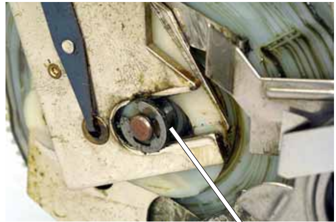
FIG. D36 Here the cam-shaft bushing is completely missing.
