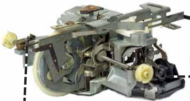
STILL-FRAME LEVER STILL-MASK CHANGEOVER ROD SPRING SPRING TAB ON SPEED-LEVER ASSEMBLY
