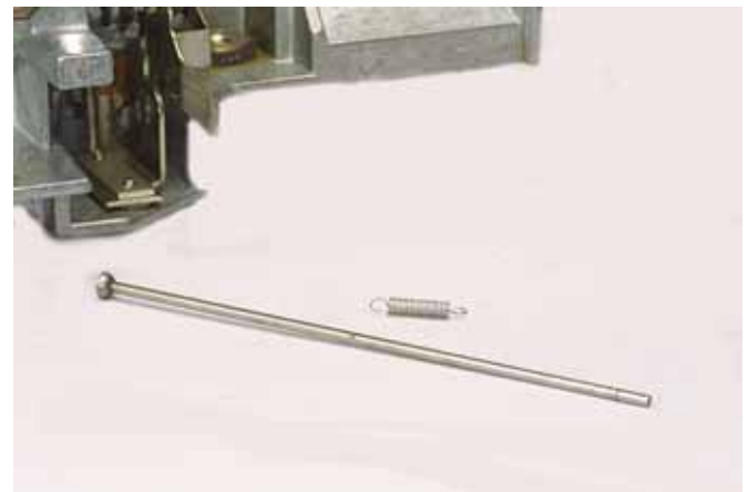
FIG. D39 Still-mask changeover rod and spring removed.
