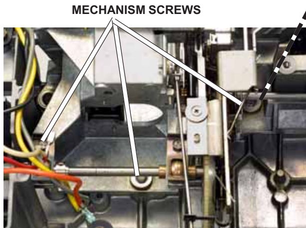
FIG. D32 Remove the three mechanism screws.
