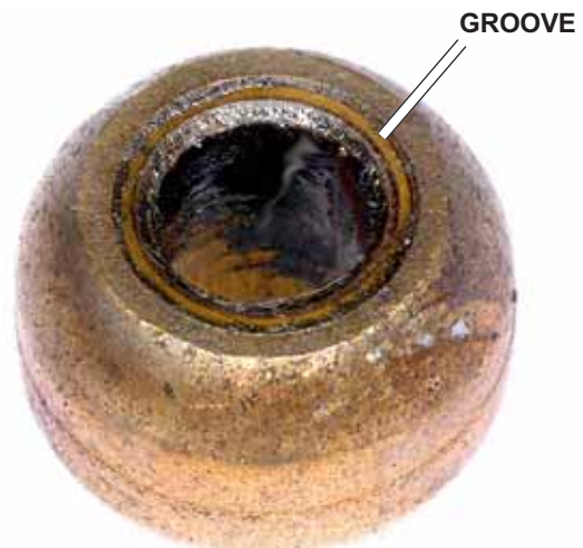
FIG. D60 The groove shows wear in the shutter-side bearing--most likely, the washer was left out.
