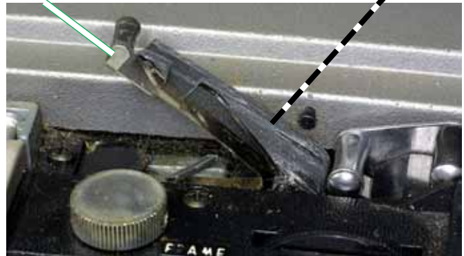
FIG. D2 A broken damping arm.
