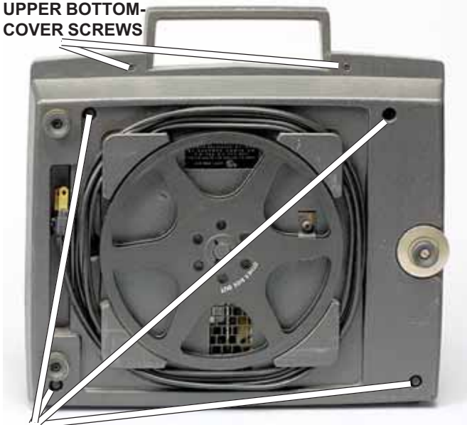
FIG. D3 Bottom of the M80 projector. Not all projectors have the two upper screws. Note that the bottom cover stores the take-up reel.
