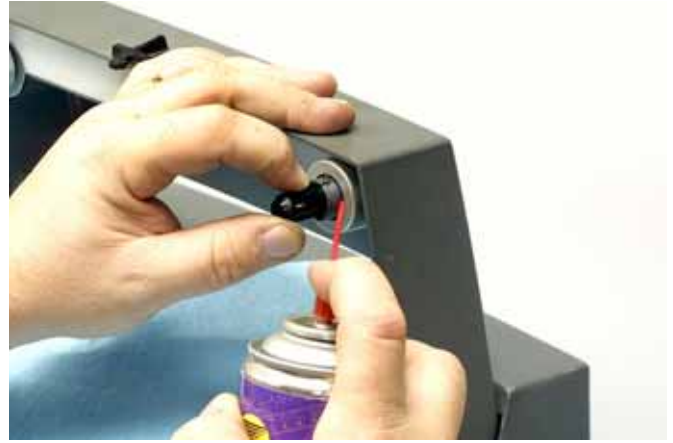
FIG. D119 Cleaning the supply spindle.
