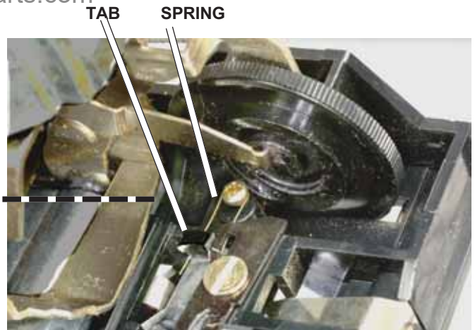
FIG. D94 Underside of damping-arm assembly.
